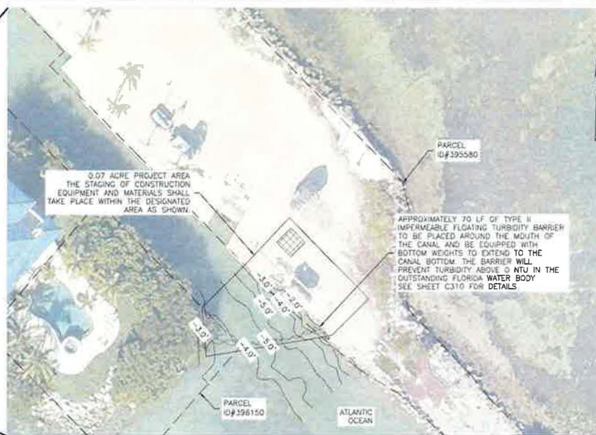
PROPOSED EROSION AND SEDIMENT CONTROL LAYOUT - WEED BARRIER
