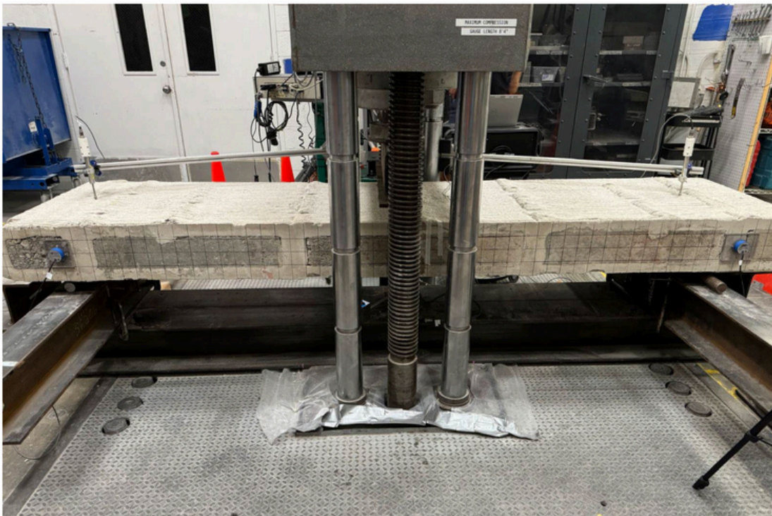
Figure 1.1 – Test setup for three-point bending of 3D Printed Slab
